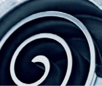
Front page: Close-up view of the inside of the scroll compressor in the Thermalia®.
